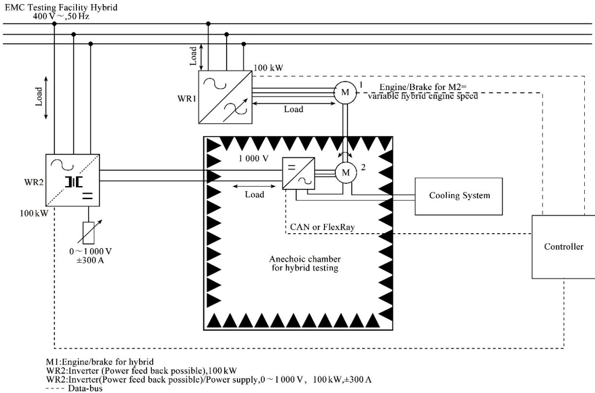
Figure 1 Basic setup of the new absorber chamber
